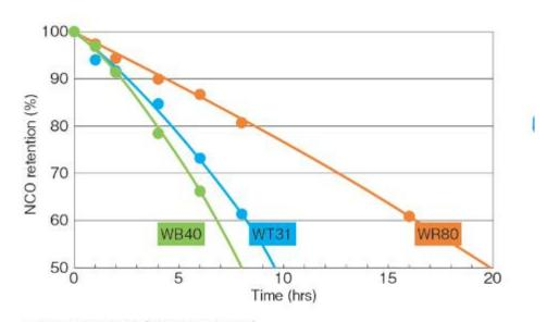
Polyol : Setaqua6520 (Nuplex Resins Ltd.) DURANATE $^{\text{TM}}$ /Polyol ratio NCO/OH=1.25 mixed and agitated 10 min. at 600rpm.
