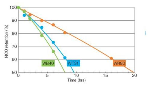
Polyol : Setaqua6520 (Nuplex Resins Ltd.) DURANATE<sup>TM</sup>/Polyol ratio NCO/OH=1.25 mixed and agitated 10 min. at 600rpm.
